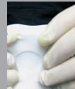
Sika® Injection-304 reacts to form a waterproof, flexible but solid polyacrylic gel.
