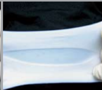
Sika® Injection-304 reacts to form a waterproof, flexible but solid polyacrylic gel.
