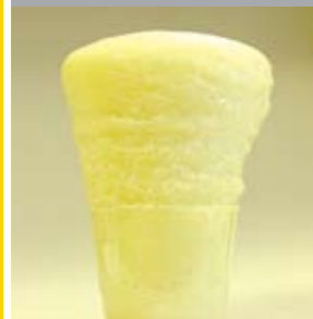
The free expansion rate of Sika® Injection-101 is up to 40 times.
