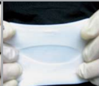
Sika® Injection-304 reacts to form a waterproof, flexible but solid polyacrylic gel.
